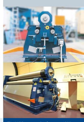
The MCS system also features, within the linear guides, large roll supports with a lubrication system able to effectively prevent wear of the bending roll.
